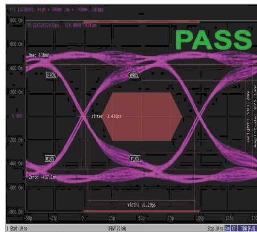
10Gb/s HDMI Eye Diagram with EZ0P33P2NA-A
